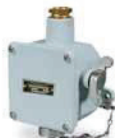
Switched interlocked sockets UNAV 1436 in marine grey painted brass with UNAV 1948 cable glands 50-60Hz IP56
