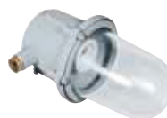
Cylindrical lighting fixtures UNAV 2132 in marine grey painted brass with UNAV 1948 cable glands 230V IP66
