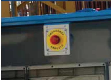
The emergency push-button located in the middle of the cabinet is always well visible and accessible even with closed lid, to guarantee the maximum safety and a quick operation.
