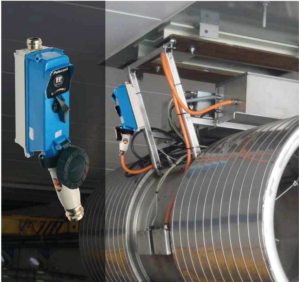
TUNNEL 54 series for electro ventilators is composed of compact switched sockets with plug in aluminium alloy. They are designed to guarantee the operating service at 400° C for 120 minutes as defined in tunnel safety regulations. Sockets are made of high resistant materials and equipped with an isolator switch of AC3-AC23A category guaranteed at rated current.
